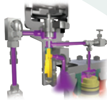
PV Valve Open (Relieving Position)
